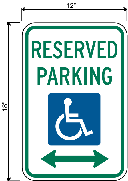
TC-P-ADA-RE-MA POLE MOUNTED ADA PARKING REGULATORY SIGN (RE-ENGINEERED) SCALE: NTS
