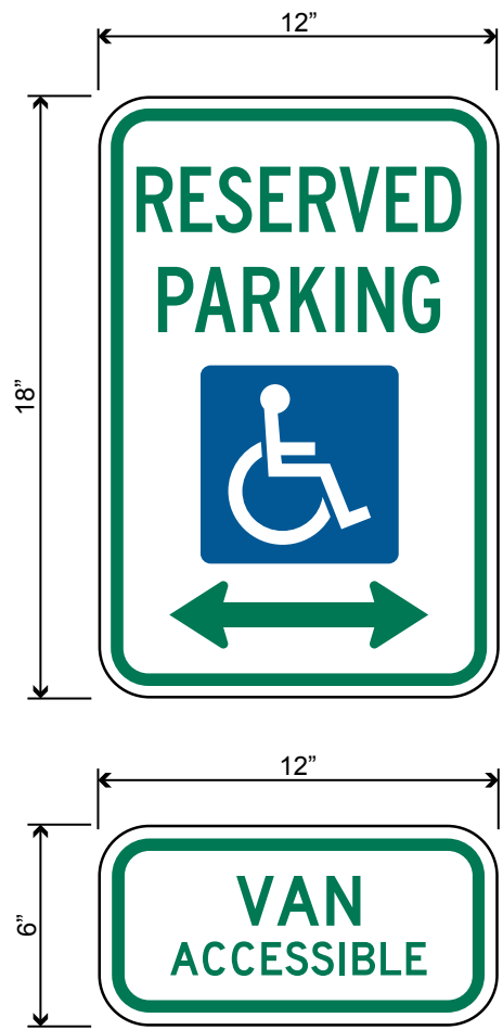
TC-P-ADA-V-RE-MA POLE MOUNTED ADA PARKING REGULATORY SIGN W/ VAN ACCESS (RE-ENGINEERED) SCALE: NTS
