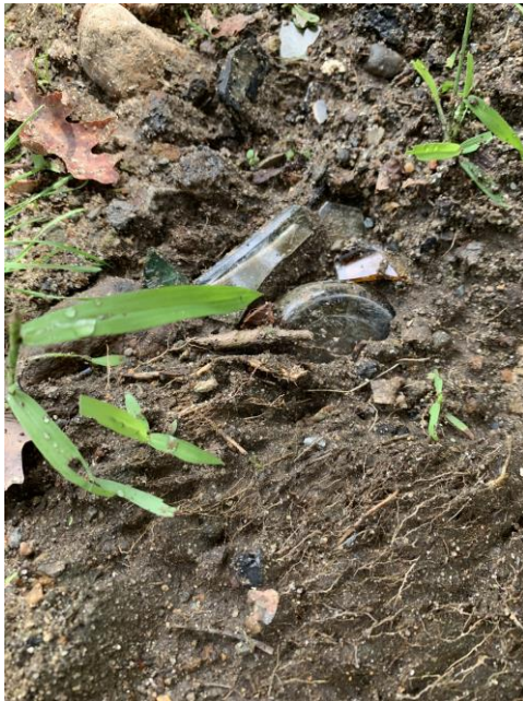
Photo 2. Glass, metal debris observed in stockpiled topsoil.
