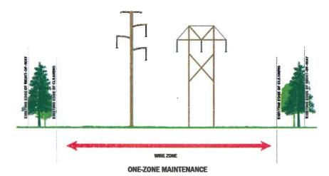
The diagram illustrates a typical right-of-way condition. This work is occurring within the existing edge of clearing. Your neighborhood may have a different configuration of transmission structures.
