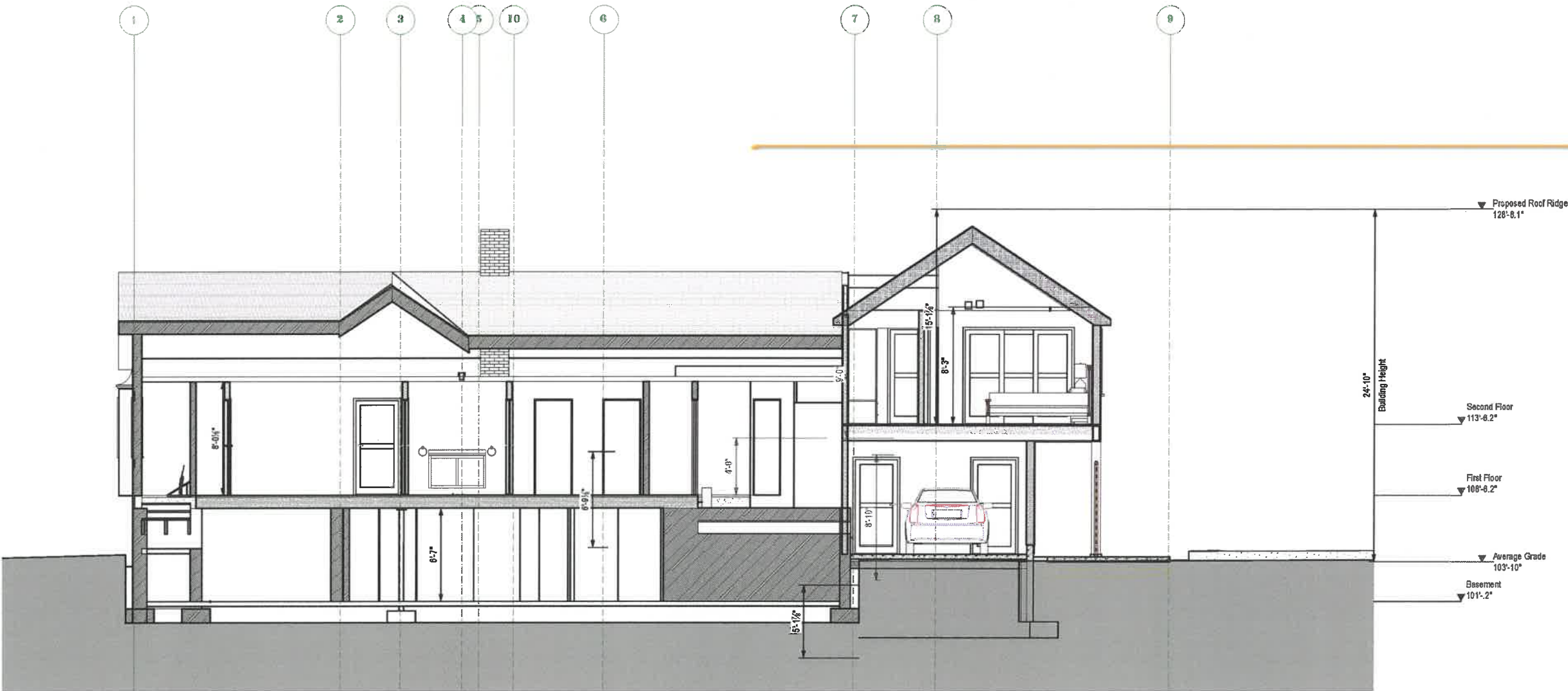
1 LONGITUDINAL SECTION : ENTRY ; LIVING ROOM; GARAGE SCALE: 1/4" = 1'-0"
